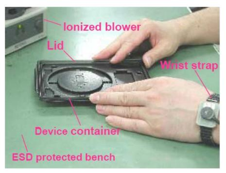
2.Place your right thumb on the corner of the packaging box cover and carefully open the box cover (applicable to APD/PIN/LD coaxial package and independently packaged optical devices).
