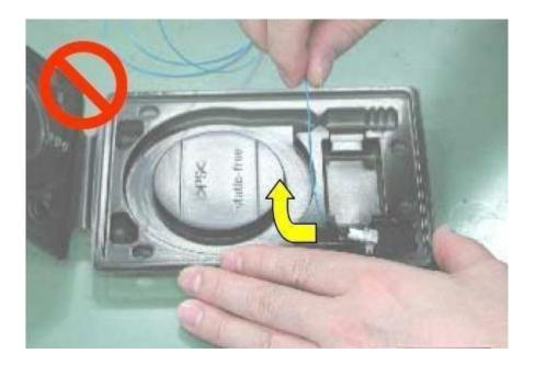
Warning: When operating optical devices, the maximum tensile force acting on the optical fiber shall not exceed 5N, and the bending radius of the optical fiber shall not be less than 35mm. Fiber damage will cause optical power to decrease. Please operate with caution!
