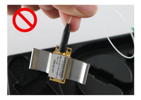
Warning: When operating optical devices, the maximum tensile force acting on the optical fiber shall not exceed 5N, and the bending radius of the optical fiber shall not be less than 35mm. Fiber damage will cause optical power to decrease. Please operate with caution!
