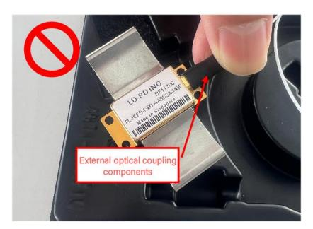
WARNING: Forces exerted on the tailbone may dislocate the optical coupling components, resulting in irreversible and permanent damage to the device!
