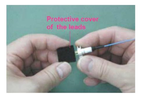
6. For butterfly-packaged devices (usually lasers), hold the opposite corners of the laser with your thumb and index finger, and carefully take it out of the packaging box.
