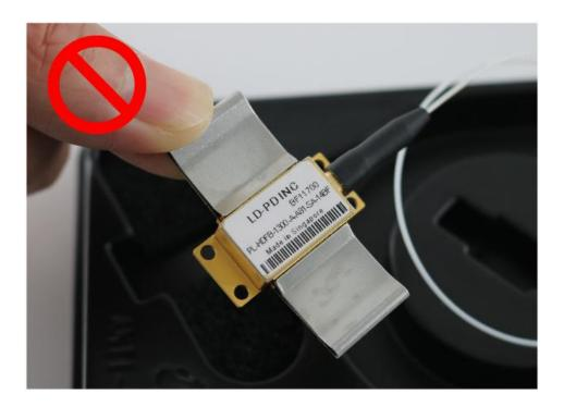
Warning: May cause deformation or damage to device pins
