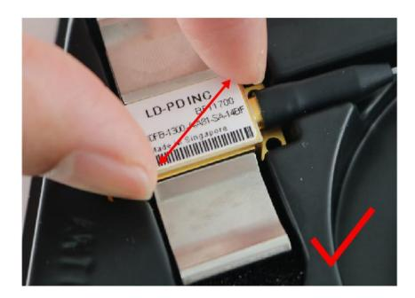
5. When grabbing the optical module product, hold the module metal box with one hand and the optical fiber and optical fiber connector with the other hand.
